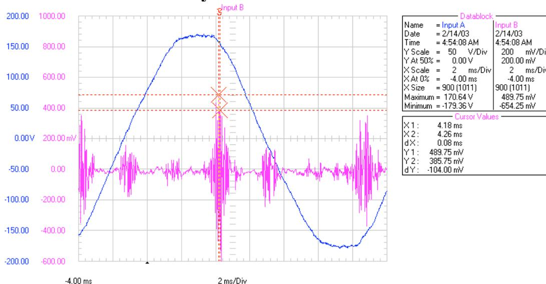
THE WAVEFORM WAS COLLECTED IN ROOM 101 OF THE BRIGHTON SCHOOL. CHANNEL 1 WAS CONNECTED TO THE UTILITY SUPPLIED 120 VAC POWER. CHANNEL 2 WAS CONNECTED TO THE SAME POTENTIAL EXCEPT THROUGH THE GRAHAM UBIQUITOUS FILTER. THE AREA BETWEEN THE CURSORS REPRESENT A FREQUENCY OF 12.5 KILO HERTZ. NO GRAHAM/STETZER SOLUTIONS FILTERS WERE BEING UTILIZED AT THE TIME. THE AMPLITUDE OF THE BURST SHOWN IS 489 MV.
